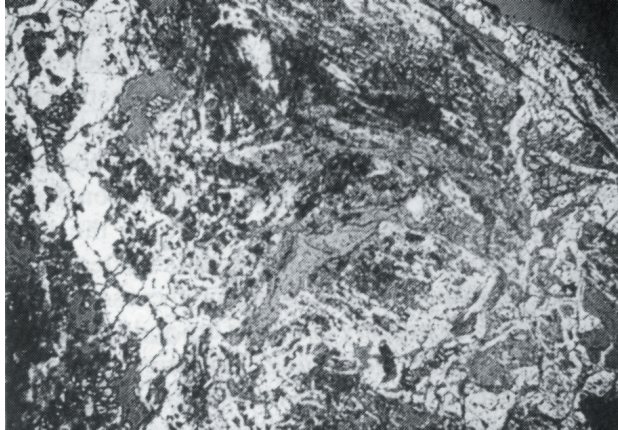
Figure 5. Remobilization and redeposition of uraninite (white mineral). Photomicrograph shows uraninite veins (left and right) partially destroyed by dissolution of uranium which has been redeposited as scattered veinlets and shapeless masses of a new generation of uraninite (middle). (Magnification 10X).
