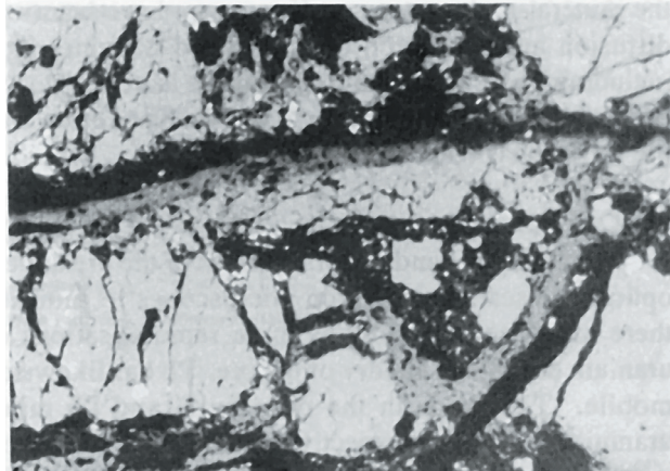
Figure 7. Two generations of uraninite grains (lighter grey), and more oxidized supergene veins and patches (darker grey). The small scattered white grains are galena. (Magnification 200X).
