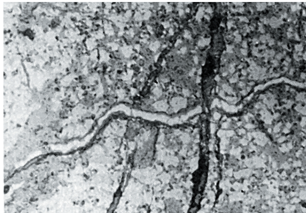
Figure 9. Remobilized uraninite (light grey) deposited as scattered grains with a chlorite (dark grey) matrix. A remobilized galena vein (white-grey) cuts across the uraninite-chlorite association. (Magnification 50X).
