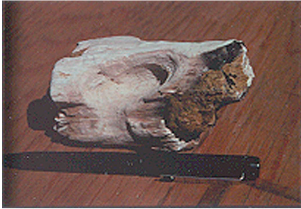
Figure 5. One of the pieces of fossilized wood recovered from the basalt flow during excavation of the upcast ventilation shaft (the pen is for scale.) The outer areas that were in contact with the hot basalt lava have been burnt to white ash. (Courtesy of B.H.P. Australia Coal Pty. Ltd.'s Crinum Mine Project.)
