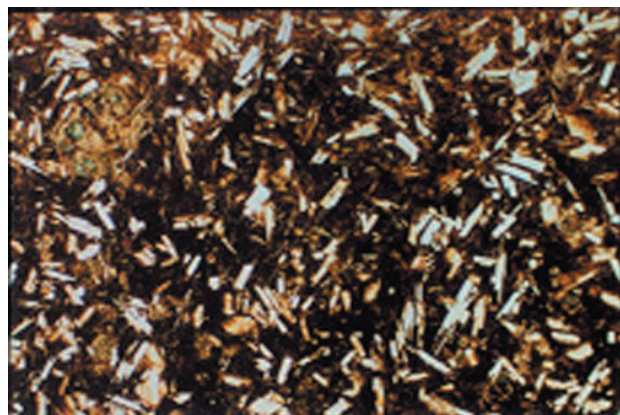
Figure 27. Polarized light photomicrograph of basalt sample BCM-3 from Drill-hole 05469 from close to the entombed fossilized wood (Figure 12). The large (1.5 mm wide) grain in the top left corner is former olivine altered to chlorite and serpentine (green), goethite (brown) and iddingsite? (blue-green). Small (0.5–1 mm long) plagioclase laths (white) are scattered uniformly through the rock, but the clinopyroxene (probably augite) between the laths has been altered to chlorite with titanomagnetite grains (black) and iron oxide staining. (Approximately 60 times magnification.)
