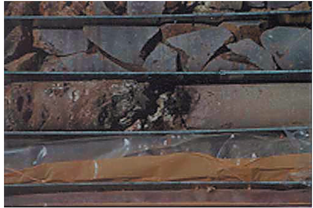
Figure 12. Drill core from Drill-hole 05469 (courtesy of BHP. Australia Coal Pty Ltd's Crinum Mine Project.) In the center of the photograph is a piece of charred fossilized wood entombed in the very bottom of the Tertiary basalt (to the left and in the next row above) right at the boundary at 25.2m with the Permian siltstone (to the right.)
