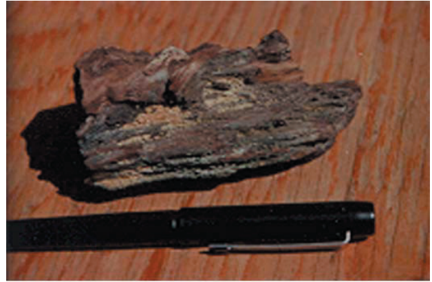
Figure 6. Another of the pieces of fossilized wood, showing black charring where it was in contact with the hot basalt lava (the pen is for scale.) Courtesy of B.H.P. Australian Coal Pty. Ltd.'s Crinum Mine Project.)
