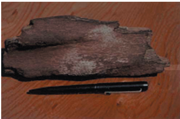
Figure 9. Another piece of the fossilized wood which shows very little charring. The fossilized wood itself is brown, probably due to impregnation with iron minerals during fossilization (the pen is for scale.) (Courtesy of B.H.P. Australian Coal Pty. Ltd.'s Crinum Mine project.)
