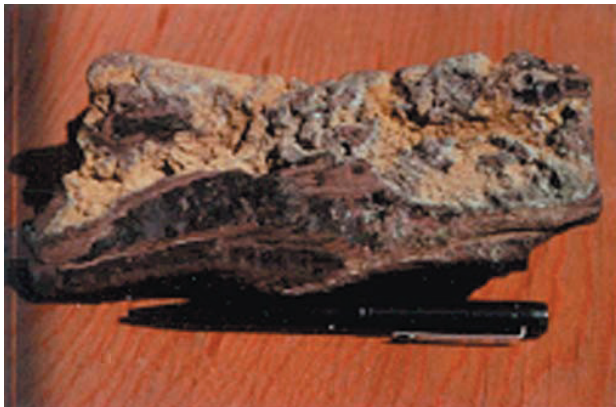
Figure 7. Another piece of the fossilized wood recovered during excavation of the upcast ventilation shaft, showing some basalt still attached to its charred outer surface (the pen is for scale.) (Courtesy of B.H.P. Australia Coal Pty. Ltd.'s Crinum Mine Project.)
