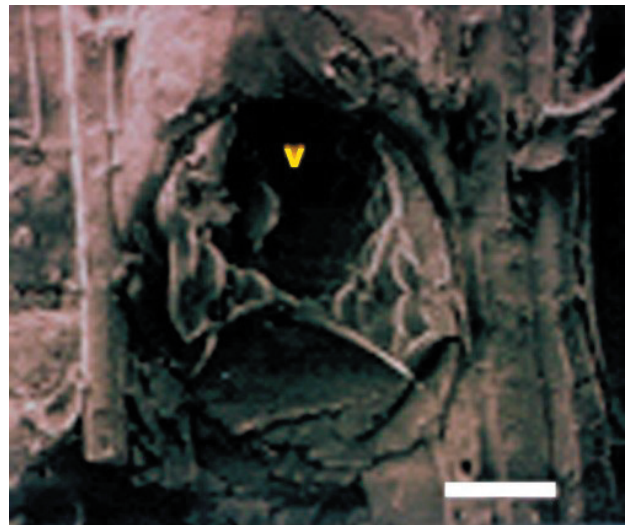
Figure 24. Field emission SEM photomicrograph of the fossilized wood showing a vessel (V) element with the remains of smooth vesicle-like structures, possibly tyloses. Bar=20mm. (Courtesy of G. Downes.)
